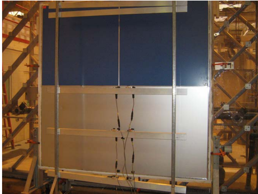
Photo No. 2 Structural Wind Load Testing
