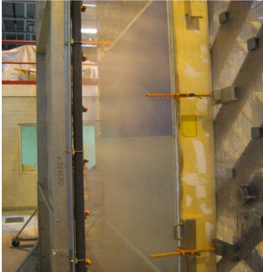
Photo No. 1 Water Penetration Testing
