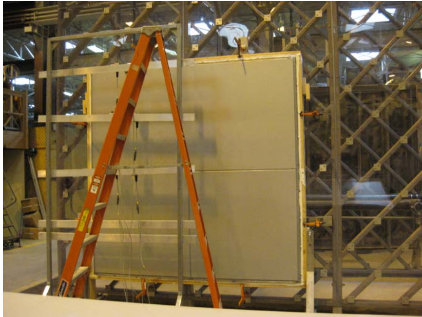
Structural Load Testing
