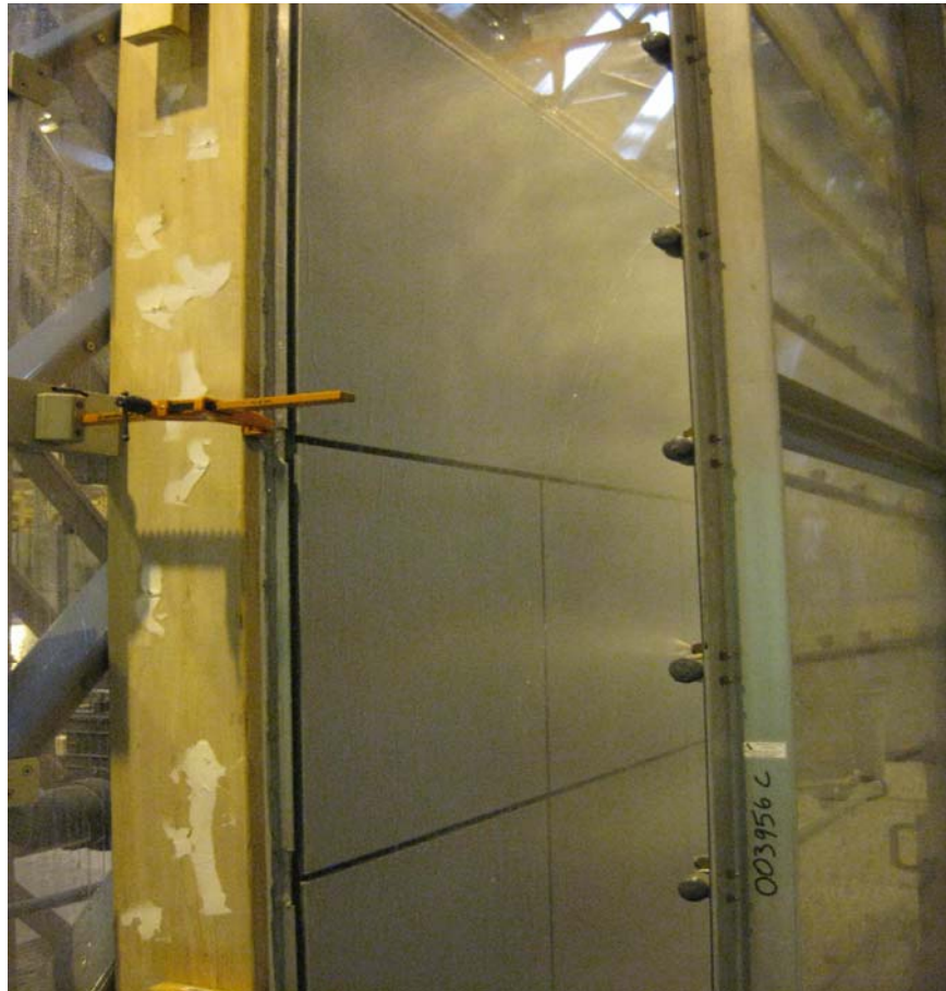
Water Penetration Testing
